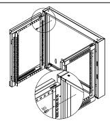
【5】 Install side frames to the grooves of back frame by 4pcs of M6\*12 screws (6pcs if more than 18U) as shown by the arrow in the picture, note 19" mounting rails are in the front side.
