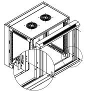
[7] Install front frame by 4pcs of M6\*12 screws (6pcs of M6\*12 screws if more than 18U), refer to the picture.
