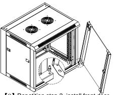
[9] Repetition step 2, install front door. Tip: SE enclosure is the bolted structure, need to adjust the diagonal size of enclosure after the assembly, ensure homogeneous space for all doors and doors work well.
