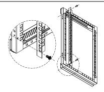
[4] Fix 19" mounting rails to the first holes of top & bottom of side frames by 4sets of M5 screws.
