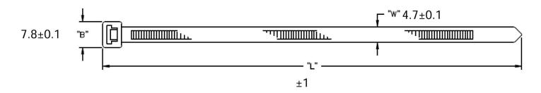
Material: UL Approved Nylon 66/94V-2, corrosion resistant, well insulation, difficult to aging.
